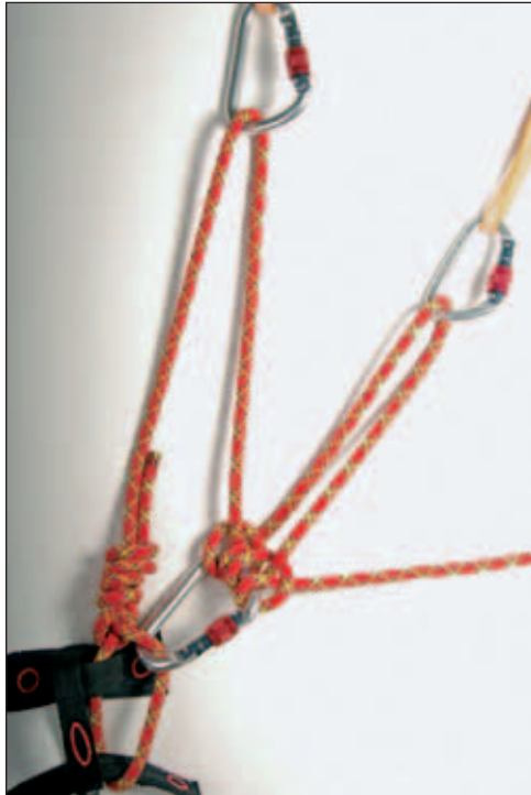
54a. Clipping into two anchors with clove hitches back to the harness.
