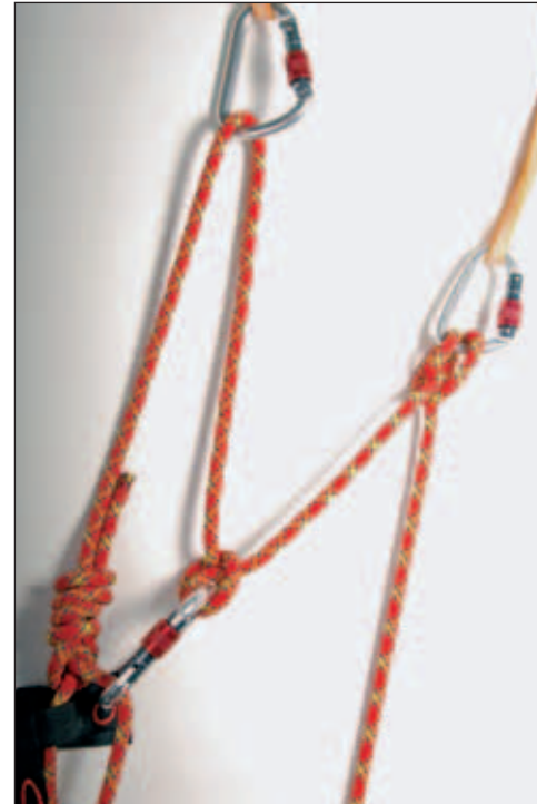
54b. Clipping directly to a second anchor with a clove hitch. Use this method only if you can easily reach the second anchor.
